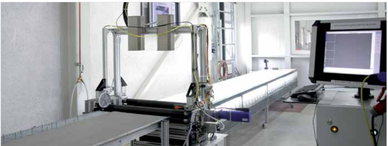
GKD's photometric inspection system
