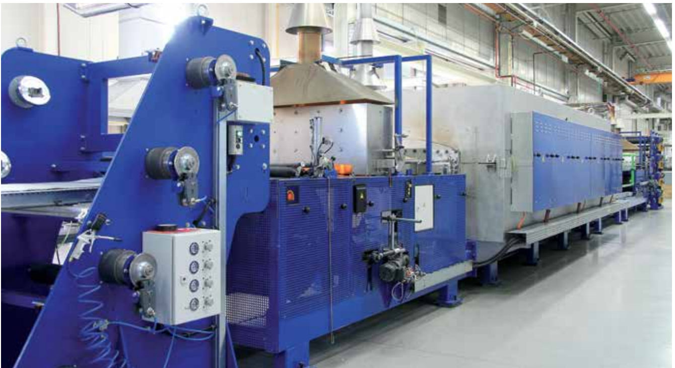
In-house API spec 6A compliant heat treatment
