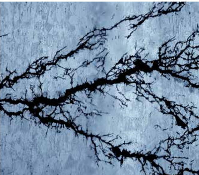
Stress corrosion Cracking (SCC)
